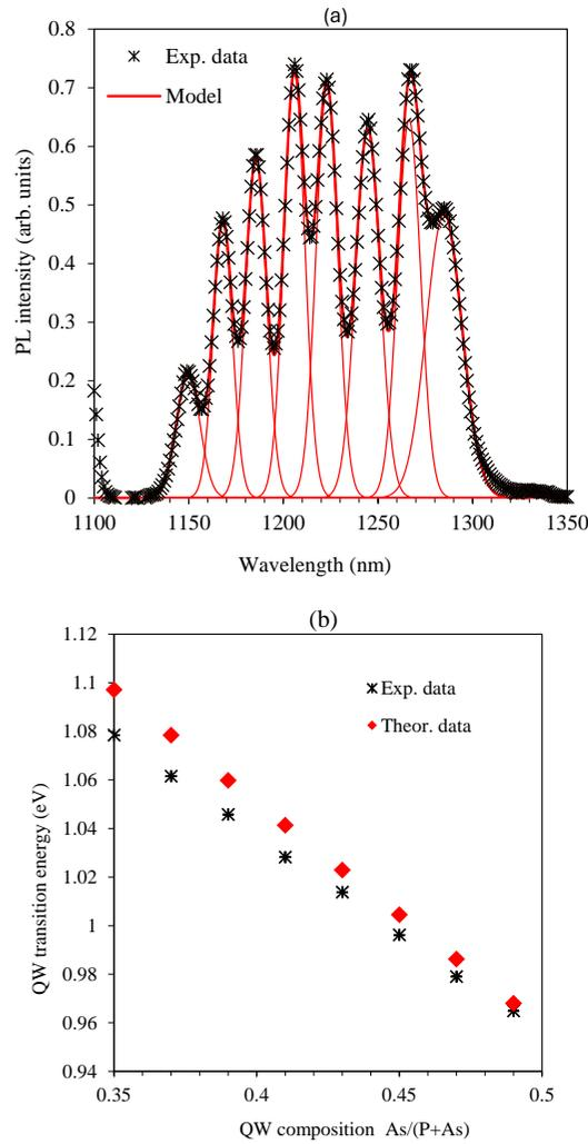
FIG. 3. (a) Low temperature (10 K) PL spectrum measured after epitaxial growth. Black symbols (\*): experimental data; red line: best-fit with the model described in the text. (b) QW transition energies versus As composition. Black symbols (\*): experimental data (PL peak energies); Red symbols (♦): calculated peak energies.
