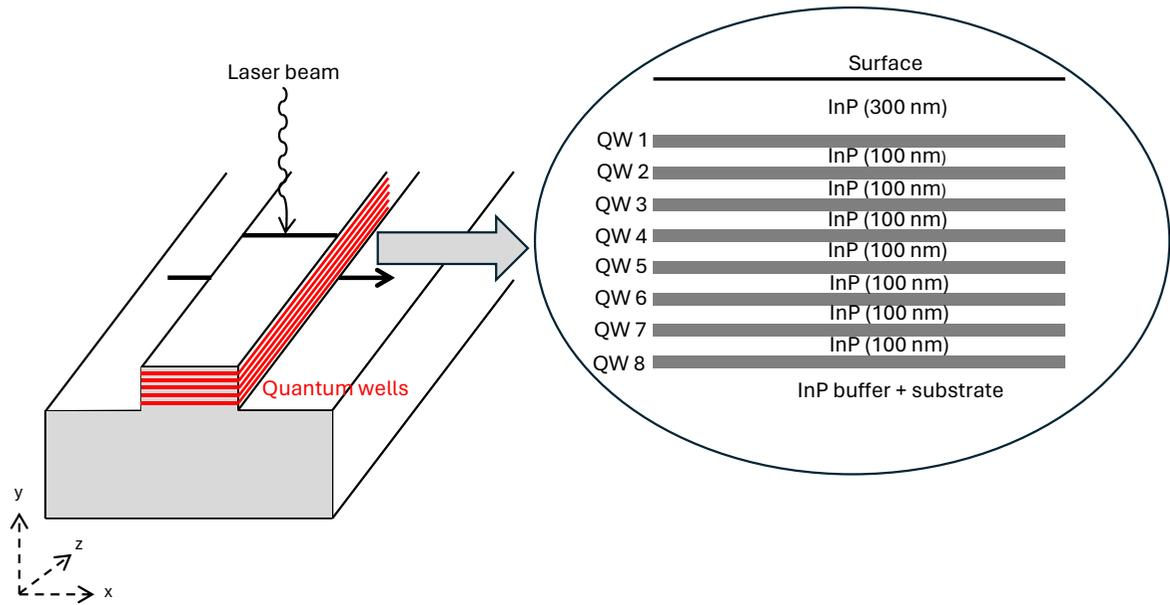
FIG. 1. Epitaxial sample structure. Each  $\text{InAs}_x\text{P}_{1-x}$  QW has the same thickness (7.5 nm). The As/(P+As) composition is step graded, from 0.49 for QW8 to 0.35 for QW1.
