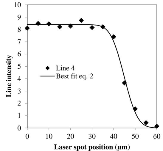
FIG. 4. Intensity profile for QW #4 as a function of the laser spot position across a cleaved edge on the reference MBE sample. The best fit curve, obtained using eq. 2, is also shown.
