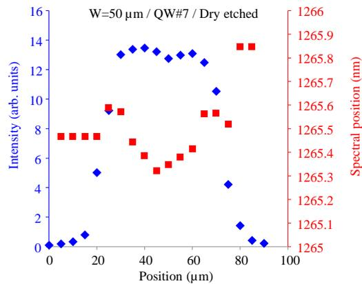
FIG. 8. Intensity profile (blue  $\blacklozenge$ ) and spectral position (red  $\blacksquare$ ) for QW #7 for a  $50 \mu\text{m}$  RIE stripe.
