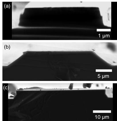
FIG. 2. Secondary electron micrographs of etched stripes, cross section. (a) Dry etched,  $\langle 0 \bar{1} 1 \rangle$  orientation, width  $5 \mu\text{m}$ . (b) Wet etched,  $\langle 0 \bar{1} 1 \rangle$  orientation, width  $20 \mu\text{m}$ . (c) Wet etched,  $\langle 0 \bar{1} \bar{1} \rangle$  orientation, width  $50 \mu\text{m}$ .
