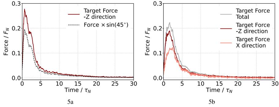
**Figure 5.** Force experienced by the target material for the vertical (left-hand panel) and oblique (right-hand panel) simulations. The sign of the force along the  $\bar{z}$ -axis has been inverted for clarity. The projection of the vertical force at  $45^\circ$  is shown in (a), for comparison with the oblique force. The amplitudes and times are normalized to  $F_N = 1.2e8$  N and  $\tau_N = 1e - 4$  s.
