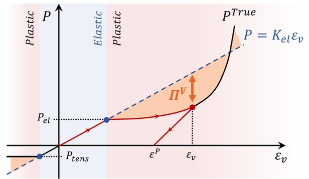
**Figure 1.** Graphic showing the computation method for volumetric stress glut. A compressed material follows a path in red in the  $\{P, \varepsilon_v\}$  space, with a pressure never exceeding  $P^{\text{True}}$  (black curve). In the orange area,  $P^{\text{True}}(\varepsilon_v)$  differs from the ideal elastic pressure  $K_{el}\varepsilon_v$  (blue curve) due to plasticity, and a volumetric stress glut  $\Pi^V$  appears.
