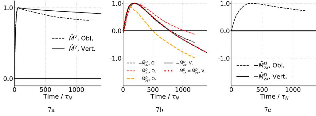
**Figure 7.** Source time functions for different parts of the moment tensor: the volumetric part  $\hat{M}^V$  (a), the diagonal terms of the deviatoric moment  $\hat{M}_{xx}^D$ ,  $\hat{M}_{yy}^D$  and  $\hat{M}_{zz}^D$  (b) and the non-diagonal term  $\hat{M}_{zx}^D$  (c). Only the non-rotated components are shown, and moments are normalized such that  $\hat{M}_{ij} = M_{ij} / \max |M_{ij}|$ .
