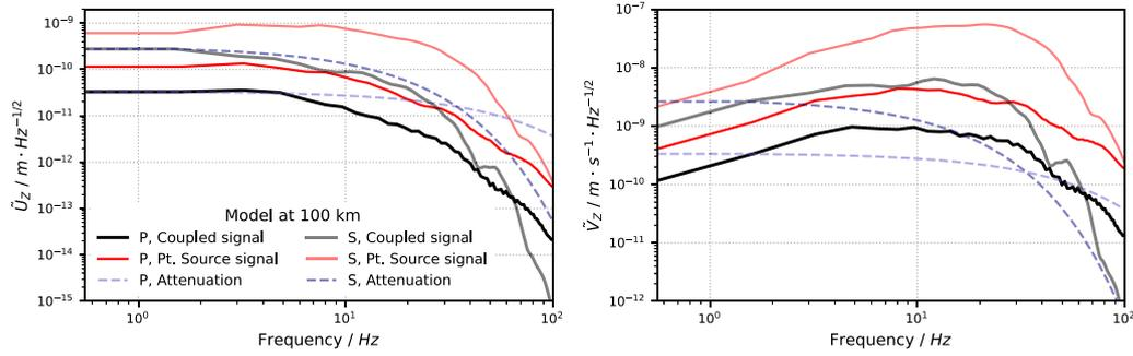
**Figure 14.** Spectra of the coupled and point-source signals extrapolated from 400 m distance up to 100 km distance, using an attenuation and crust model from (Garcia *et al.* 2022). The right-hand plot represents vertical displacement and the left-hand plot vertical velocities of the *S* and *P* waves. The attenuation spectra is represented with dashed blue lines.
