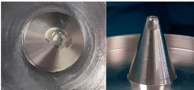
(a) acceleration nozzle (b) Collection nozzle
