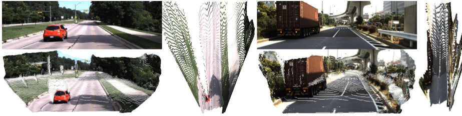
Fig. 9: Point cloud reconstructions on the previously unseen DDAD dataset. The view-point of the bottom point cloud is translated 2m up and 8m back, while the side one is a top-down view. We can see that even though some artifacts are present, the overall shape and geometry of the scene is preserved.
