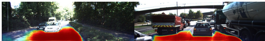
Fig. 6: Example of segmentation quality of ground attention. Even in cases where there are close obstacles, the attention stays precise.
