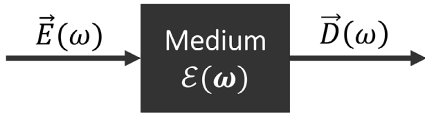
Figure 1. The linear dielectric permittivity of a material is defined in the constitutive relations by a transfer function linking the output displacement field \vec{D} to the input electric field \vec{E} . It shares the properties of a linear transfer and can be analytically expressed using the singularity expansion method.
