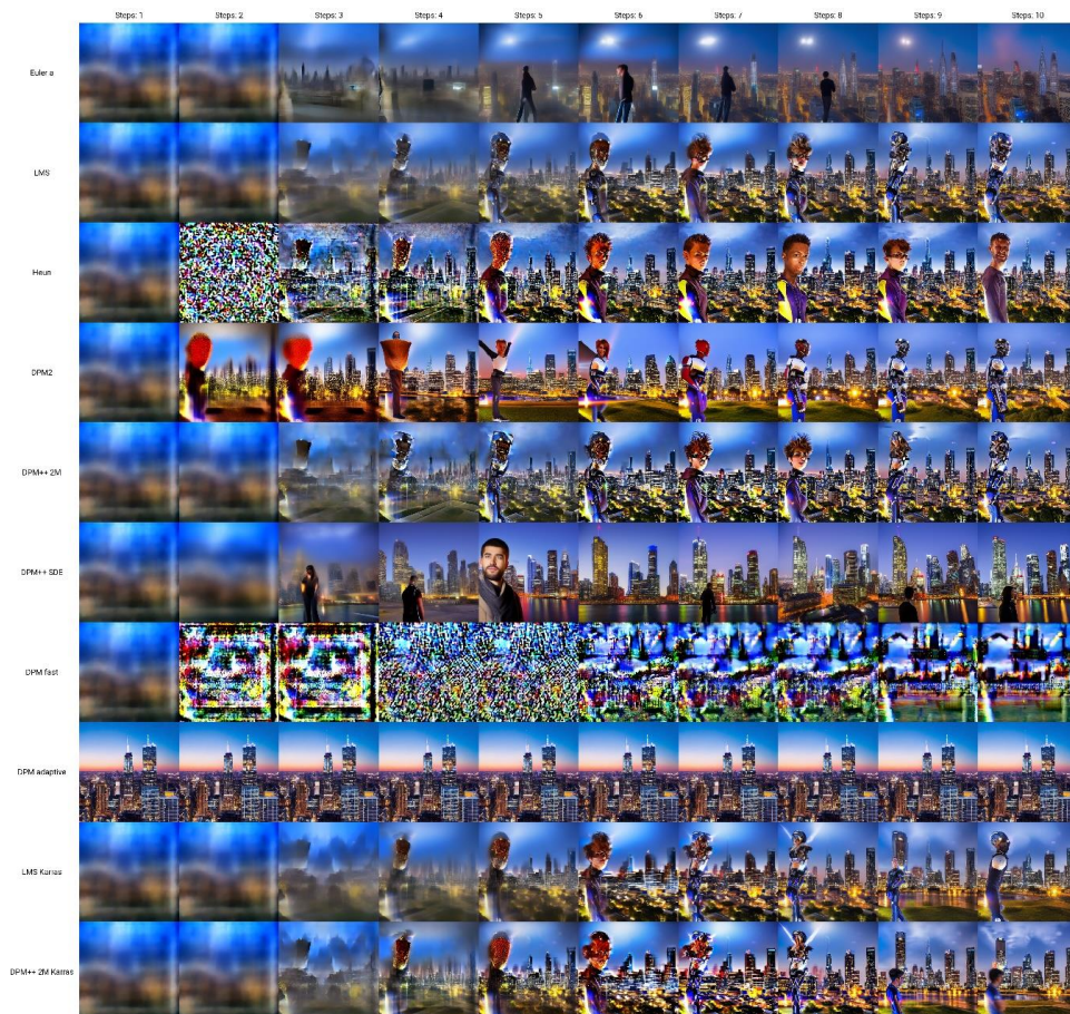
Fig. 4: An illustration of how Stable Diffusion uses noise removal to produce an image. This example shows the model’s response to the prompt ‘Hyperrealistic photo portrait wide shot of a cyborg, city background’ enacted in 10 steps, using 10 different sampling methods (aka samplers), from ‘Euler a’ through to ‘DPM++ 2M Karras’. Each sampler has its own way of applying noise reduction to obtain an image.
