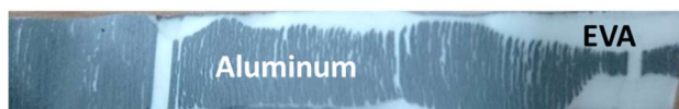
Fig. 11. Photograph of a peeled specimen of the EVA interface with the rear side of the cell, with aluminium visible on its surface.
