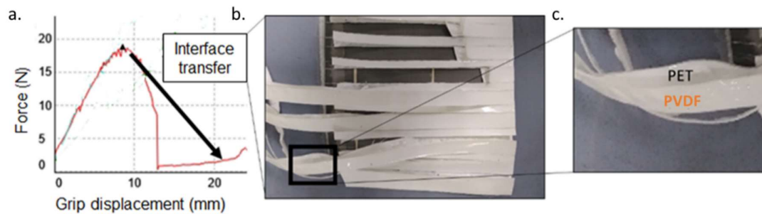
Fig. 18. (a) Effect of interface transfer on the peel curve. (b) Photograph of a sample with an internally separated backsheet and (c) an expanded view of the area inside the black rectangle, showing the separation at the PET/PVDF interface.
