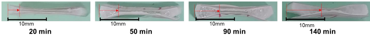
Figure 6: Interface advance of the front of diffusion over time (example for backsheet/EVA/backsheet samples)
