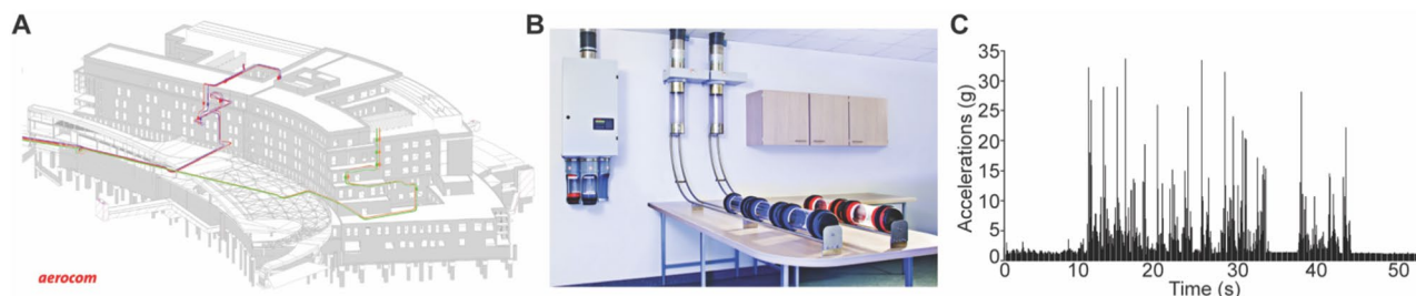
Figure 1. Characterization of the pneumatic transportation system (PTS). (A) Map of the PTS at the Institut de Cancérologie Strasbourg Europe. In red the one used for this study. (B) Representation of the setup used for transportation of the monoclonal antibodies (mAbs). (C) Characterization of the cumulative (x, y, and z axis) acceleration forces applied to the mAbs.
