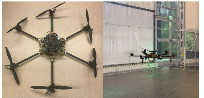
Fig. 4: The figure shows, on the left, the Tilthex platform which was used in the experiments. Note the propeller tilt angles which allow full actuation of the platform. While the image on the right shows the Tilthex executing the optimized full pose trajectory
