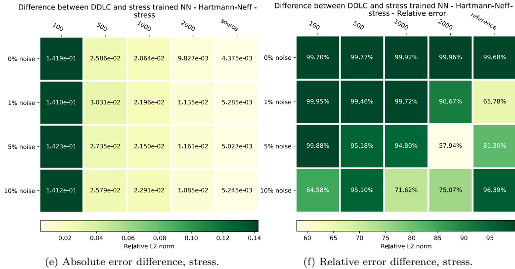
Figure 14: Relative L^2 norm error difference between DDLC and NN approaches for Cook's membrane with Hartmann-Neff law. Figures in the left column show the absolute differences between the errors, whereas those in the right column show the respective relative errors.
