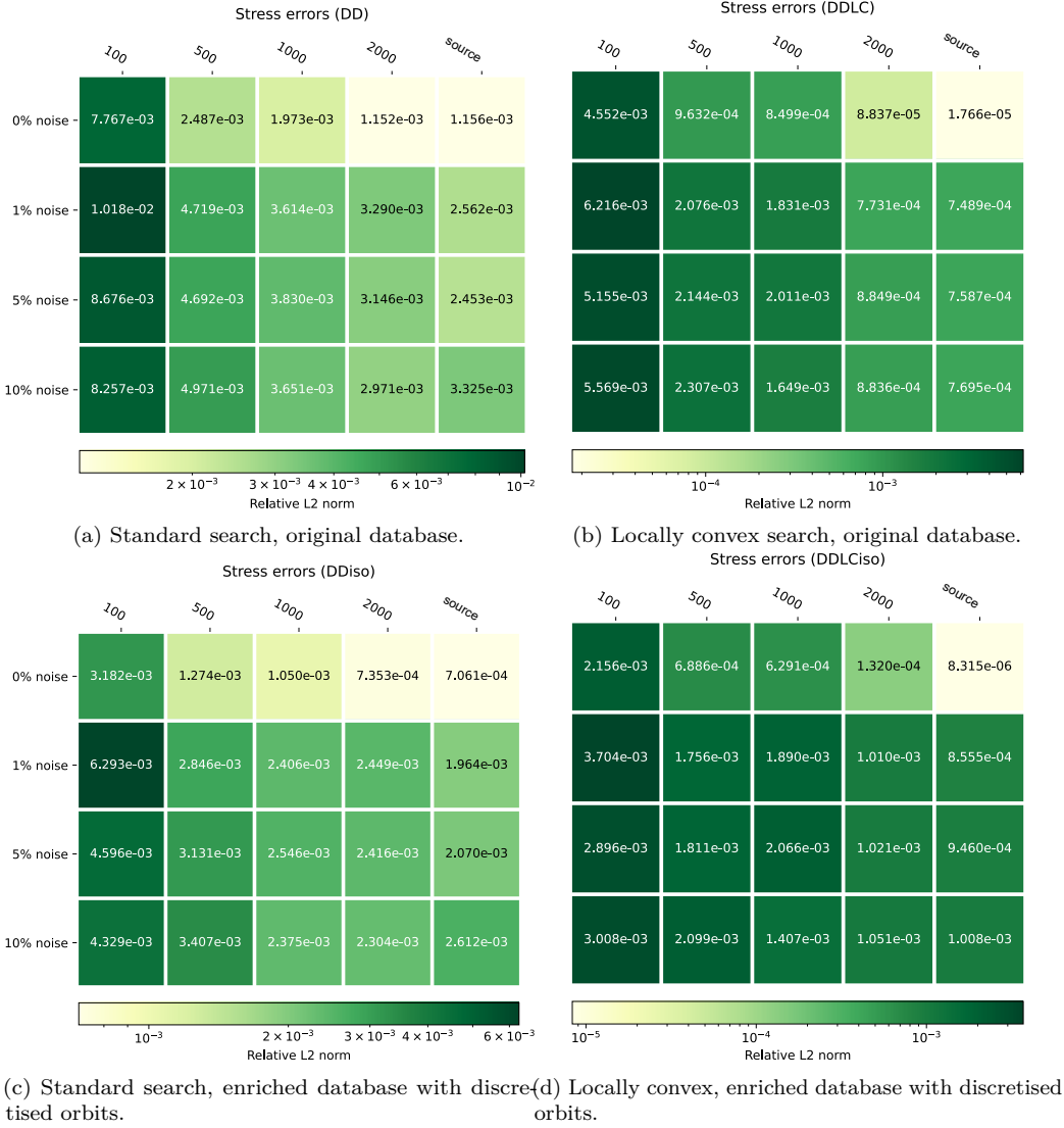
Figure 4: Relative L^2 norm of stress for Cook membrane with Ciarlet law for DDCM procedures.
