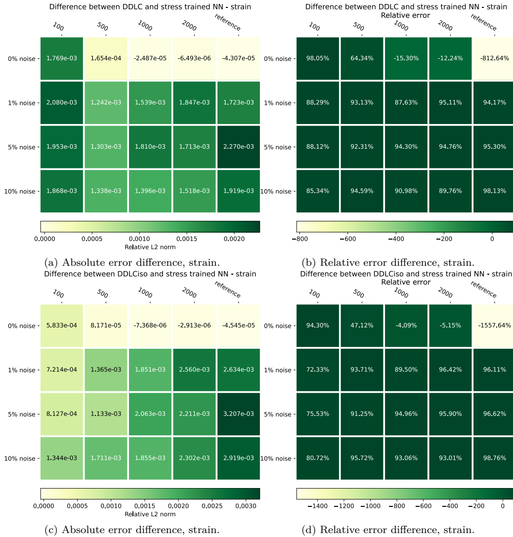
Figure C.23: Relative L^2 norm error differences between DD and NN approaches for Cook's membrane with Ciarlet law, strain. The upper row shows the absolute error difference and relative error when comparing DDLC to stress trained NNs, while the bottom row shows the errors when comparing DDLCiso to stress trained NNs.
