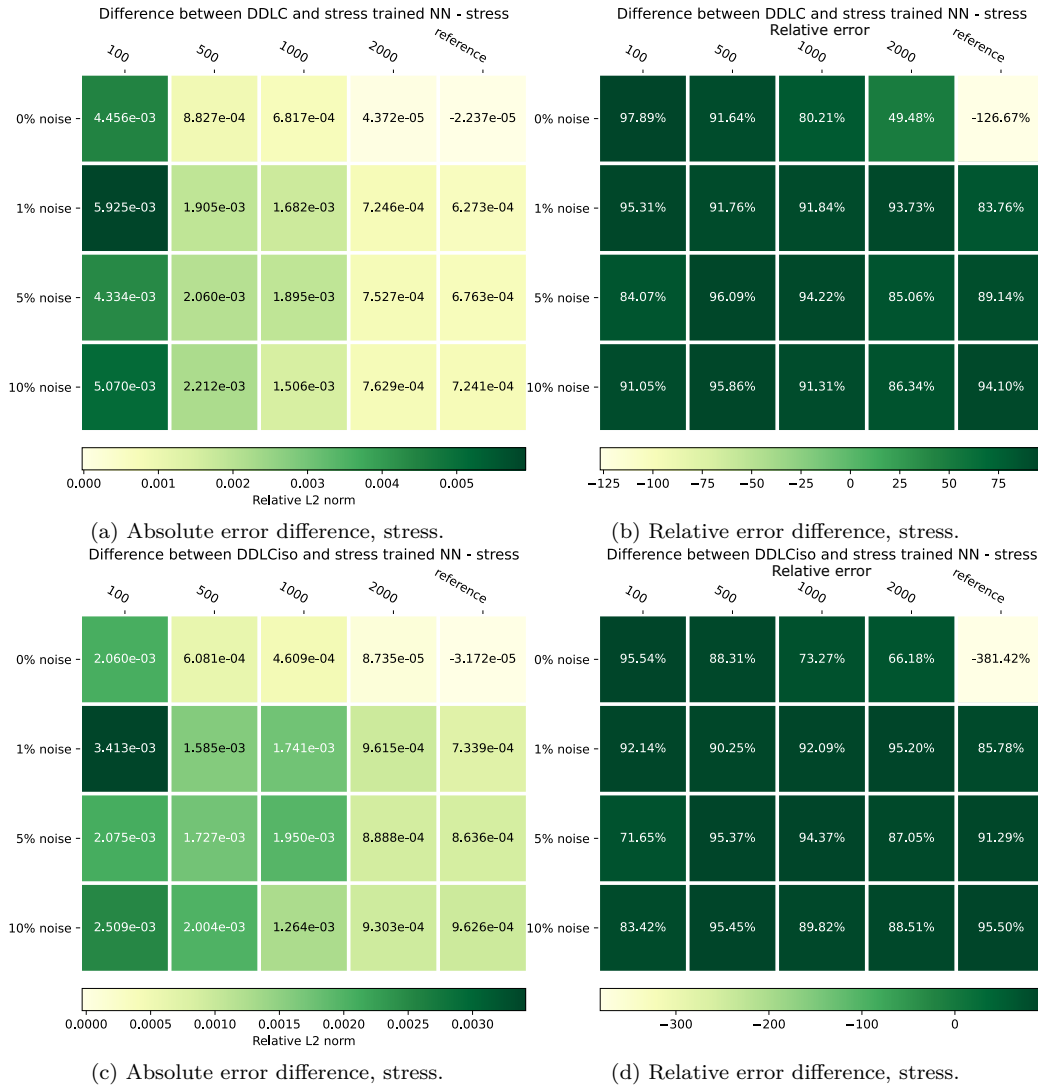
Figure C.24: Relative L^2 norm error difference between DD and NN approaches for Cook's membrane with Ciarlet law, stress. The upper row shows the absolute error difference and relative error when comparing DDLC to stress trained NNs, while the bottom row shows the errors when comparing DDLCiso to stress trained NNs.
