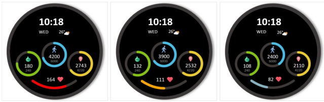
Figure 1: Examples of three watch-face stimuli showing the three radial progress charts: calories burned (cb) , step count (sc) , and distance walked (dw) . The visualized progress percentage on each stimulus are: cb: 75% , dw: 70% , sc: 65% (left), sc: 65% , dw: 60% , cb: 55% (middle), and dw: 50% , cb: 45% , sc: 40% (right).
