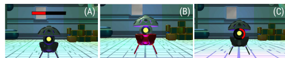
FIGURE 6: (a) Non-integrated design: a horizontal bar chart positioned outside of the robot; (b) Fully-integrated design: a vertical bar chart integrated into the texture of the robot; and (c) Partial-match design: a circular bar (donut) matching a part of the robot's shape.
