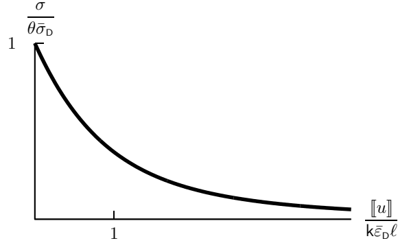
Figure 8: Graph of the cohesive law obtained for n = 1 which gives \sigma in term of \llbracket u \rrbracket . Note that the curve is monotonically decreasing, but tends only asymptotically to 0.
