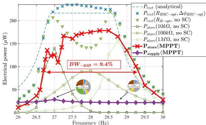
**Fig. 18.** Electrical power as a function of the input frequency. Theoretical and extracted power with discrete R (blue), experimental harvested power with a fixed and optimal  $R_{DC/DC}$  (green curves) and experimental harvested power with the proposed MPPT and RSC interface (red) as well as the power consumption of the system (purple). Pie charts are the ones of Fig. 17 ( $DC_{TLCM} = 13\%$ ).
