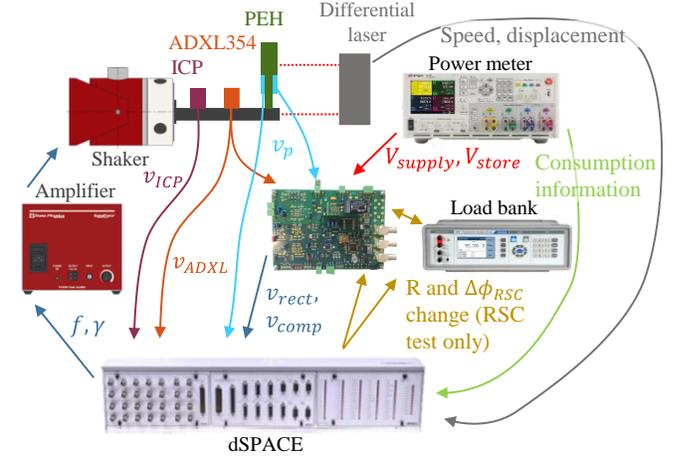
**Fig. 14.** Representation of the experimental setup used for vibration testing: RSC interface testing (test board with load bank) and autonomous mode (test board only). Other laboratory equipment is for monitoring purposes only.
