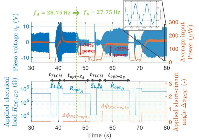
**Fig. 16.** Example of measured waveforms for the proposed architecture (MPPT + RSC interface). PEH voltage  $v_p$  and harvested power on  $V_{store}$  (top plot), as well as applied parameters  $R_{DC/DC}$  and  $\Delta\phi_{RSC}$  (bottom plot), as a function of time, if the input frequency is reduced from 28.75 Hz to 27.75 Hz ( $DC_{TLCM} = 30\%$  for greater figure clarity).
