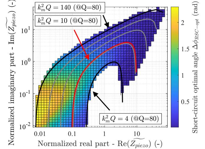
**Fig. 6.** 50x50 map of short-circuit angle versus normalized impedance  $\widetilde{Z}_{piezo}$ . Lines for specific values of  $k_m^2 Q$  are drawn on top of the map. Background color is equivalent to  $\Delta\phi_{RSC-opt} = 0$  rad. Characteristics of our harvester, presented in section V, are shown in red.
