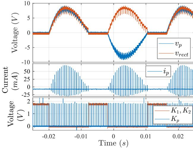
**Fig. 8.** Measured voltage and current waveforms of the RSC interface at  $f_{input} = 27.5$  Hz with  $R_{DC/DC} = 100$  k $\Omega$  ( $t_{on} = 10$   $\mu$ s,  $f_{DC/DC} = 2$  kHz) and  $\Delta\phi_{RSC} = 1$  rad
