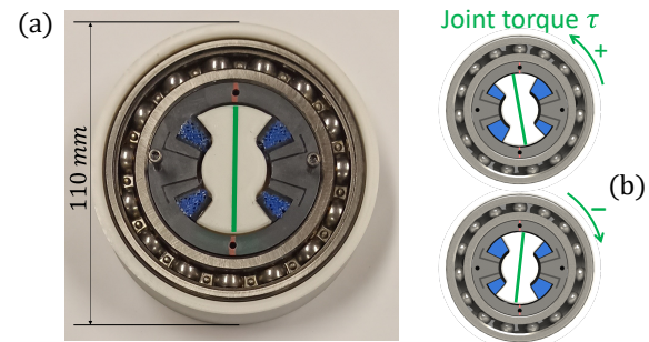
Fig. 1. (a) Picture of the proposed torque sensor. (b) Behavior under torque: for a given torque direction, two deformable capacitive structures are compressed while the other ones are relaxed.
