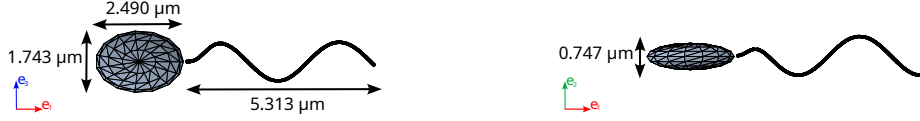
FIG. 9. Optimal swimmer, in frame (e_1, e_3) (Left) and in frame (e_1, e_2) (Right), according to the inverse efficiency (16) from [8] by optimizing only the radius of the ellipsoidal head. The geometric parameters are presented in Table VII.
