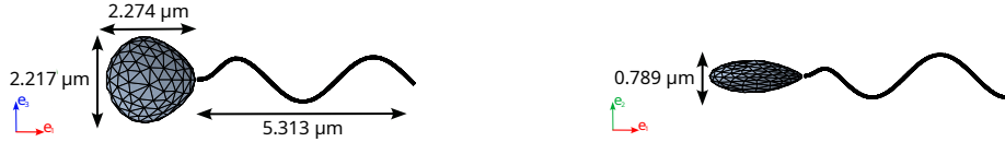
FIG. 14. Optimal swimmer obtained by the head optimization of the literature swimmer from [8] in the frame (e_1, e_3) (Left) and in the frame (e_1, e_2) (Right).
