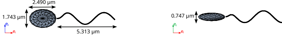
FIG. 9. Optimal swimmer, in frame (e_1, e_3) (Left) and in frame (e_1, e_2) (Right), according to the inverse efficiency (16) from [8] by optimizing only the radius of the ellipsoidal head. The geometric parameters are presented in Table VII.
