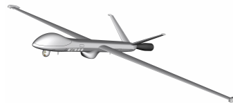
Figure 1: A fixed-wing unmanned aerial vehicle (UAV) is a large drone remotely operated.
