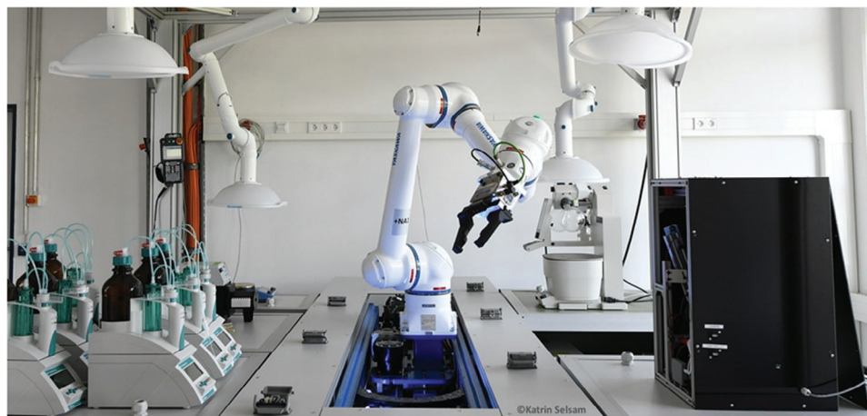
Figure 4. One of the robotic platforms (located at Fraunhofer ISC) developed in BIG-MAP utilizing a pluggable module system where each module is dedicated to a specific task like dosing, mixing, heating, evaporation and phase separation. A six-axis robot in the center of the platform integrates the modules and handles the material and container transport between them. (Reproduced with permission. Copyright 2024, Fraunhofer ISC.).
