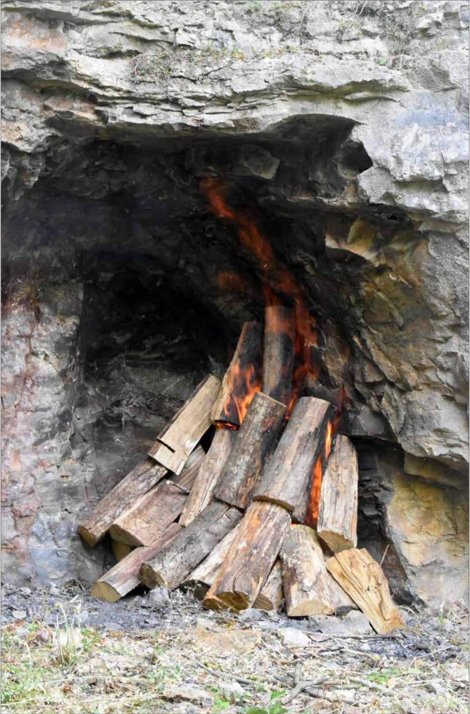
Figure 5. Pyre mounted on the working face.
