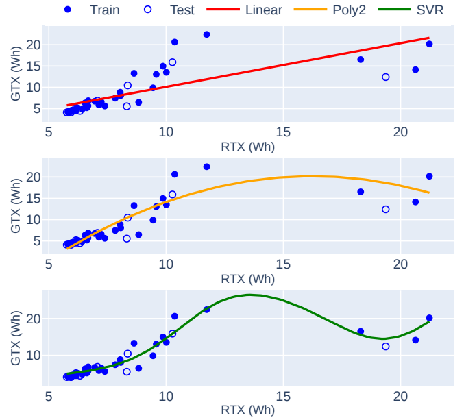
Fig. 4: Illustration of different regression types to model the energy consumption of the RTX-GTX hardware pair.
