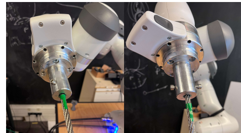
Fig. 4: Fixation of the cable before (left) and after the manipulation (right)
