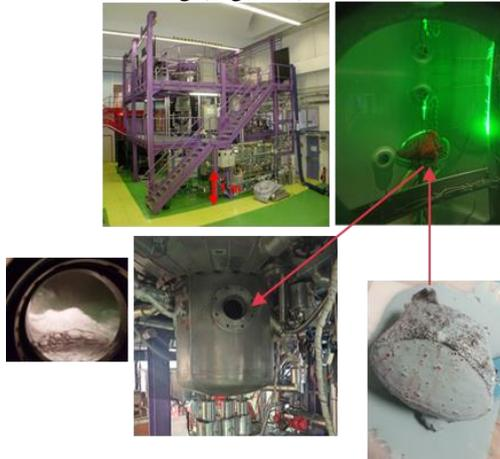
**Fig. 5: View of the TOSQAN facility used to study the resin coating efficiency for underwater conditions due to various stresses – IRSN Saclay**
