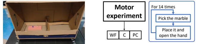
Fig. 7. Setup of the motor experiment, using Without Feedback (WF), Proprioception Contact Feedback (PC) and Contact Feedback (C).
