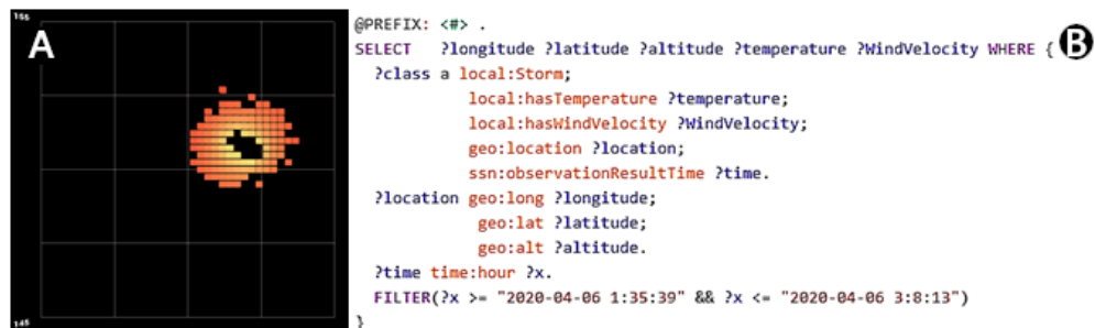
Fig. 3 A) Data points resulting from “Storm Zone” voice command. B) The corresponding SPARQL query to find all data points (individuals) belonging to the inference class Storm during a specific interval of time.
