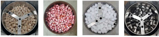
Fig. 4. Mockup drums modeled in MCNP. From left to right: wood–PVC–polyethylene–stainless steel.
