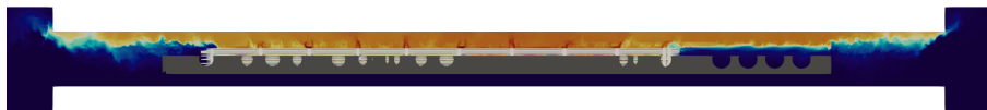
Figure 6: Temperature field for one evaluation of the CFD model (in this view, the cart has been cut for the sake of visibility).
