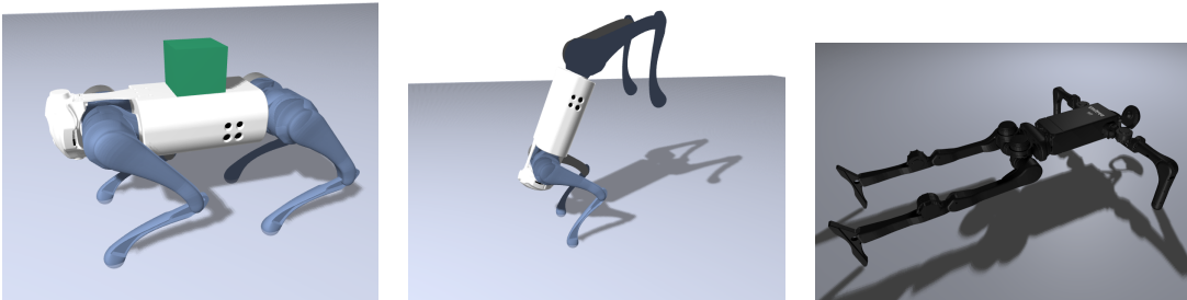
Fig. 6. The differentiable simulator is used to find a control torque stabilizing various robotics systems: a Unitree Go1 in a standing position with a 10kg mass on its back (Left) or in a "hand-stand" pose (Center) and a humanoid Unitree H1 in a "push-up" pose (Right).
