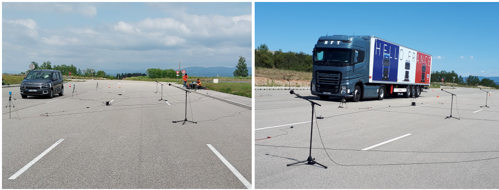
Figure 1: Controlled pass-by experiment with a light vehicle (left) and an heavy vehicle (right)
