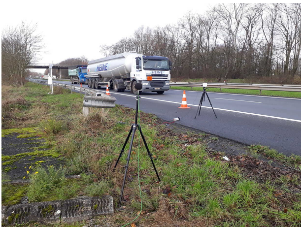
Figure 4: Left: Pass-by set up according to ISO 11819-1:2002 procedure. Right: Example of regression analysis between L_{A,max} and passing-by vehicles speeds
