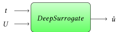
Figure 2: A deep neural network takes as input a time step t and velocity U . It outputs a prediction \hat{u} , corresponding to the discretized velocity field of the fluid.
