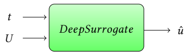
Figure 2: A deep neural network takes as input a time step t and velocity U . It outputs a prediction \hat{u} , corresponding to the discretized velocity field of the fluid.
