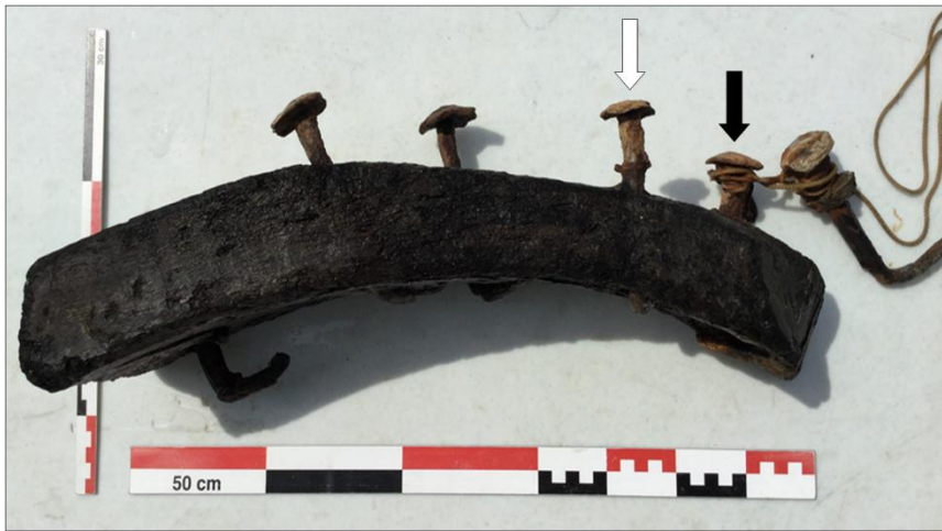
Figure 1. Hull timber fragment extracted from the wreck n°2 Courbiac-Saintes-Fontcouverte. The wood samples were cut around the nail indicated by the white arrow. The black arrow indicates the analyzed nail.
