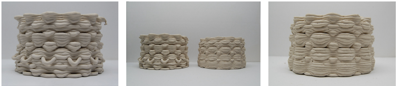
Figure 7: With clay, we 3D-printed cylinders encoded with compressed and filtered accelerometer data. The first day of recording, in November 2021 on the left and the last day of recording in June 2022 on the right.
