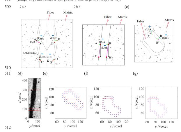
513 Fig. 15 Analysis diagram of normal and tangential displacement jumps in the *xOy* plane.
