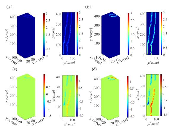
433 Fig. 11. Strain fields. Maximum principal strain when F = 126 N (a) and F = 161 N. Shear strain 434  $\mathcal{E}_{xz}$  when F = 126 N (c) and F = 161 N (d).
