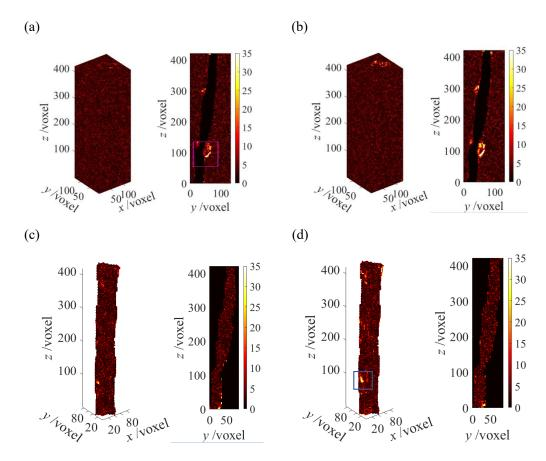
404 Fig. 9 Gray-level residual fields. In the matrix when F = 126 N (a) and F = 161 N (b); 405 in the fiber when F = 126 N (c) and F = 161 N (d).
