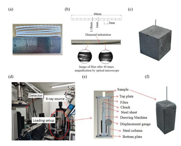
Fig. 1 Specimens and Experimental setup. (a) Polypropylene fibers. (b) Structural diagram and
