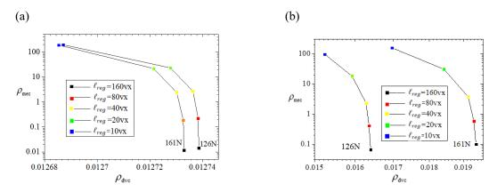
Fig. 7 Mechanical residual  $\rho_{mec}$  and correlation residual  $\rho_{dvc}$  under different loads and regularization lengths. (a) Matrix. (b) Fiber.
