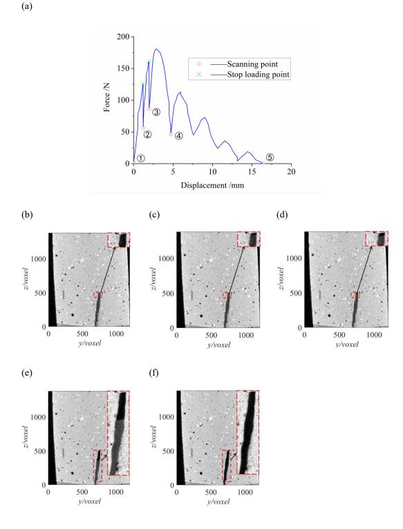
Fig. 3 Force-displacement curve for the in-situ pullout test and middle sections of steps 1 to 5.
