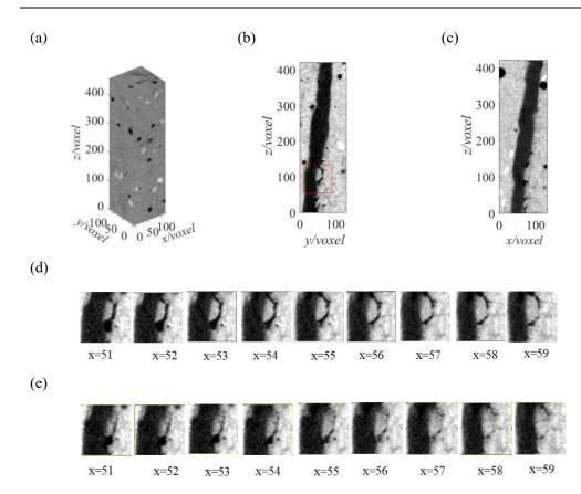
Fig. 4 Effect of fiber pullout on the matrix. (a) DVC calculation region (VOI). (b) *yOz* sections at
