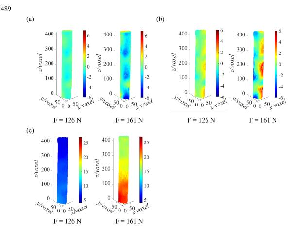
Fig. 14 3D renderings of displacement jump fields for the normal (a), tangential (b) andlongitudinal (c) components.
