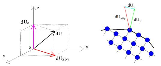
451 Fig. 12. Decomposition dU into z-direction and normal and tangential displacement jumps in the 452 xOy plane.
