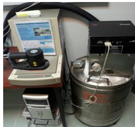
Fig. 1. The TA Instruments Q2000 DSC device was employed for conducting differential enthalpy analysis [8].
