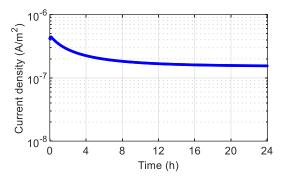
Fig.2 Simulated current density vs. time when no ions are accounted for, for a 200  $\mu$ m-thick XLPE polarized at 30 kV/mm during 24h at 25°C.
