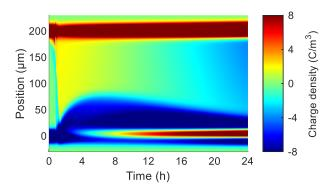
Fig.5 Simulated net charge density as a function of time and space when ions and electronic charges are accounted for. Mobility of positive and negative ions are respectively :  $10^{-14}$  and  $10^{-18}$  m<sup>2</sup>.V<sup>-1</sup>.s<sup>-1</sup>.
