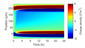
Fig.3 Simulated net charge density as a function of time and space when ions only are accounted for, for a 200  $\mu$ m-thick XLPE polarized at 30 kV/mm during 24h at 25°C.
