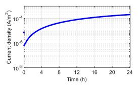
Fig.4 Simulated current density vs. time when ions only are accounted for, for a 200 μm-thick XLPE polarized at 30 kV/mm during 24h at 25°C.
