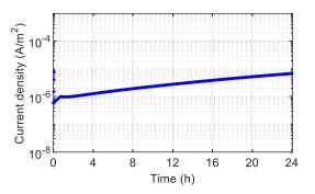
Fig.6 Simulated current density vs. time when ions and electronic charges are accounted for. Mobility of positive and negative ions are respectively :  $10^{-14}$  and  $10^{-18}$  m<sup>2</sup>.V<sup>-1</sup>.s<sup>-1</sup>.
