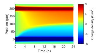
Fig.1 Simulated net charge density as a function of time and space when no ions are accounted for, for a 200  $\mu$ m-thick XLPE polarized at 30 kV/mm during 24h at 25°C.
