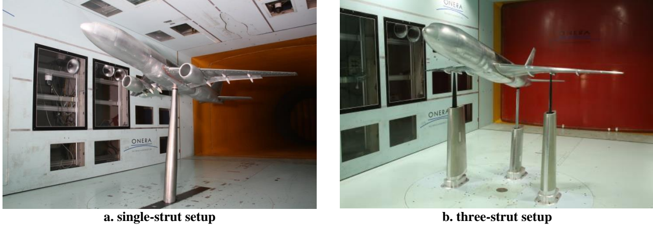
Figure 1: LRM-HL model in F1 wind tunnel
