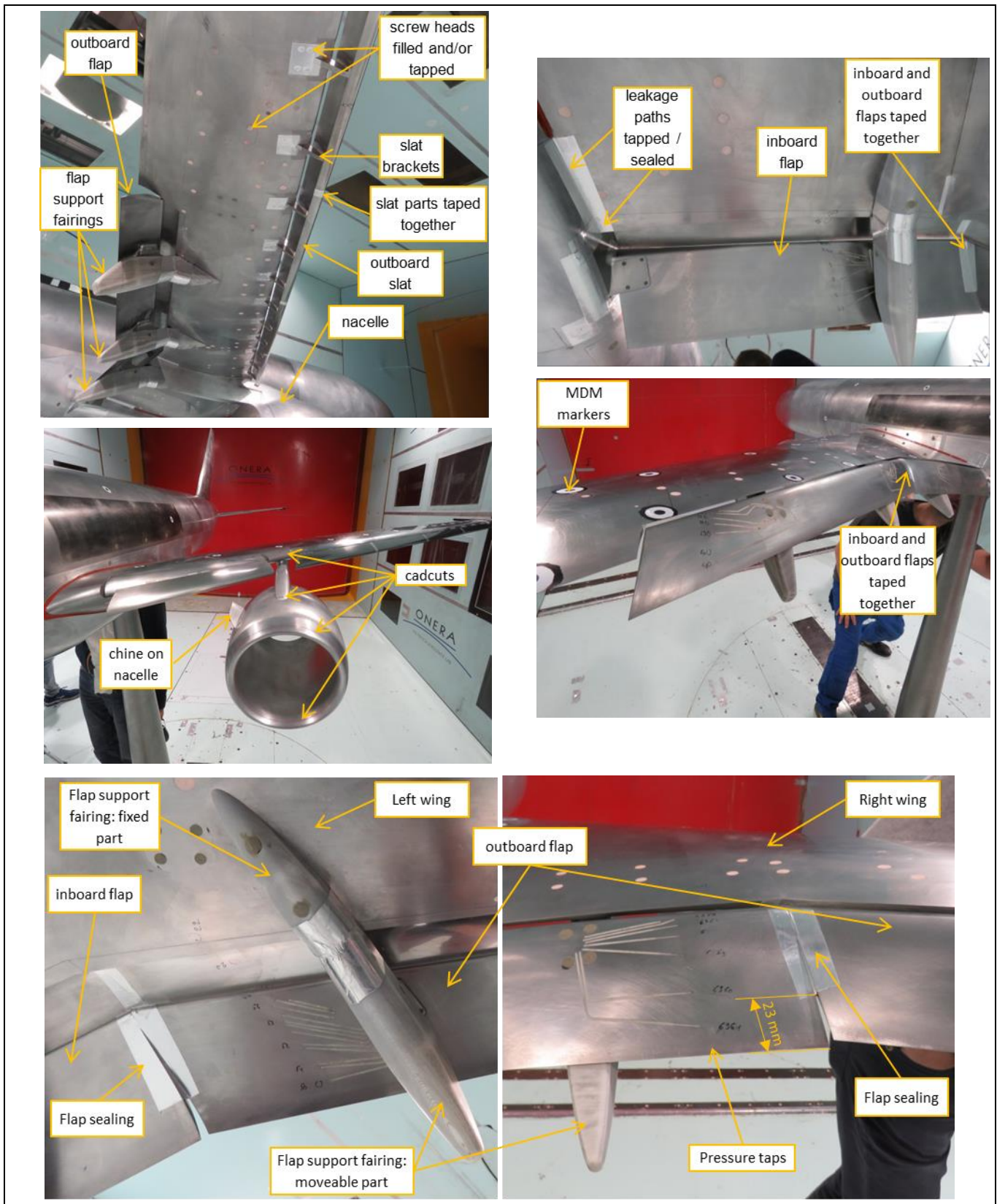
Figure 2: Details of the wind tunnel model in LDG configuration.
