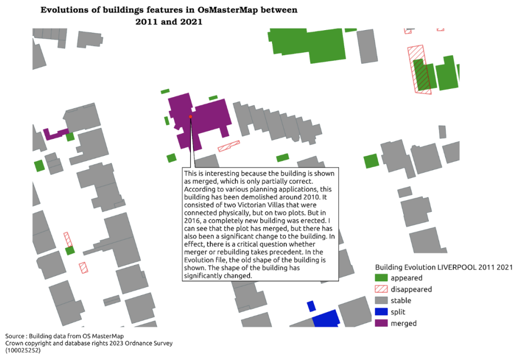
Figure 2. Example of Geospatial User Feedback on the building evolution model, with change detection on OSMasterMap 2011 and 2021 data for Liverpool.
