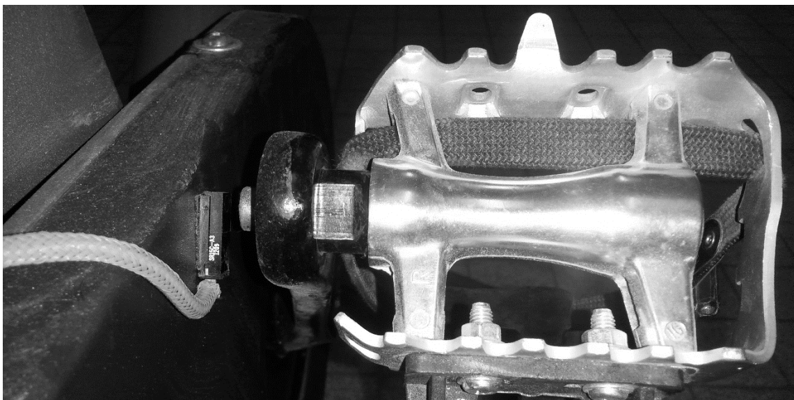
Figure 4. Magnet attached to the pedal and Hall-effect sensor attached to the ergocycle frame.
