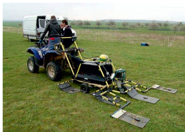
Figure 4. Electrostatic resistivity meter with two depths of investigation for soil mapping at large scale (from [19]).
