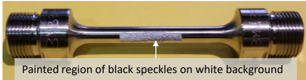
FIG. 3. Dogbone tensile specimen of SLM IN718 with speckle pattern for DIC. The white paint increases contrast and eliminates glare, and the black paint provides the speckles for tracking displacement.
