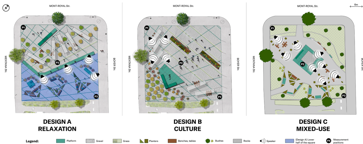
Fig. 1. Map of the studied site, showing each of the design layouts (Design A and B: 2018; Design C: 2019), as well as measurements and speaker positions. Maps for designs A and B provided by design firm Castor et Pollux and used and edited with permission.
