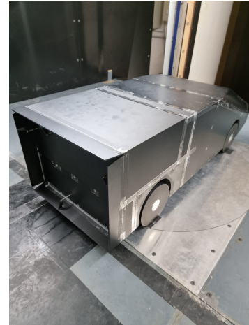
Figure 1: Windsor body equipped with the four actuated flaps on the rear.
