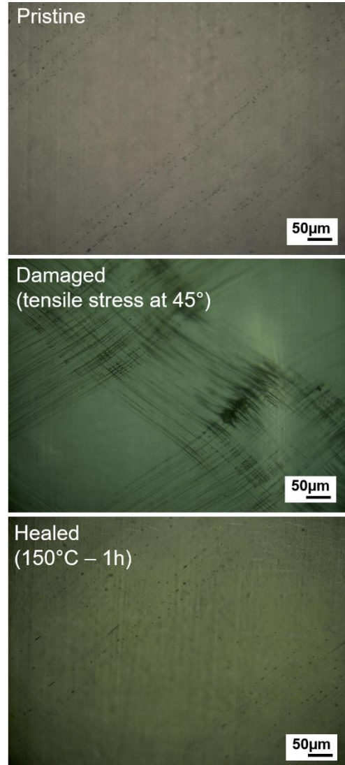
FIGURE 11. Qualitative demonstration of healing composite material after creating interfacial defects (tensile stress at a 45^\circ angle from the reinforcement orientation).
