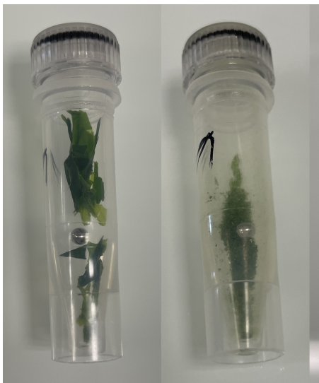
Example of dry algae with 3 mm steel ball before and after grinding process in individual tube
