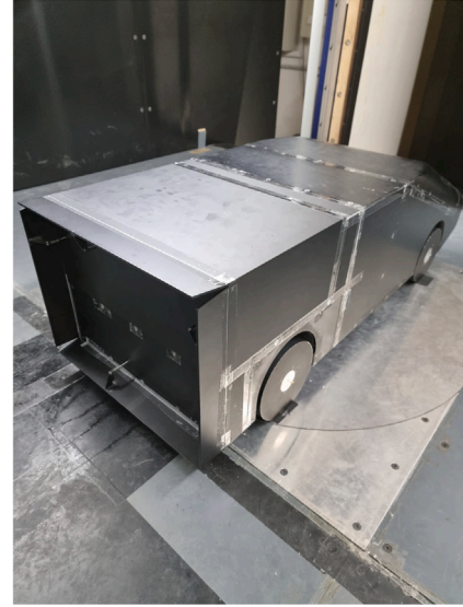
Fig. 1. Windsor body equipped with the four actuated flaps on the rear.
