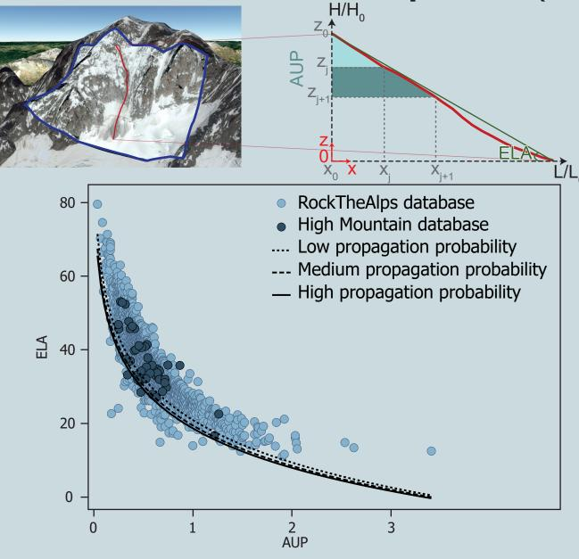
\*2 Angle between the maximum drop heigh and the maximum horizontal deposition distance (from the top of the scar to the tip of the deposit)
