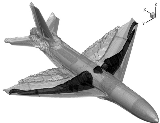
Fig. 15. Far-field integration volumes for CDvp (grey) and CDw (black); WBHV without surface roughness; overset grids; S1MA conditions; Ma = 0.85 , Re = 4.65 \times 10^6 , \alpha = 2.50^\circ .
