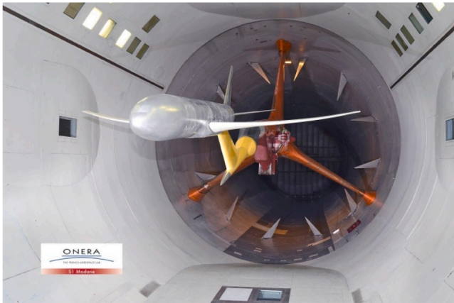
Fig. 8. S1MA model with PSP on the wings in the wind tunnel test section.
